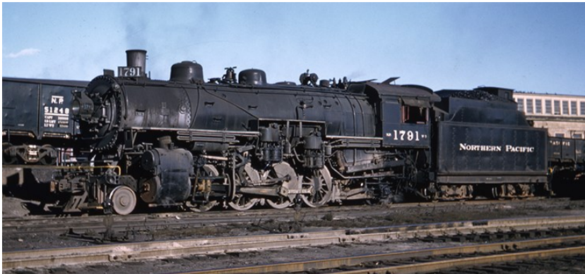
NP 1791, a Class W-3 2-8-2 steam locomotive, at Duluth in 1957. The 2-8-2s handled general merchandise trains, coal trains, and iron ore trains and made the majority of steam powered long-haul freight runs between the Twin Ports and Twin Cities. (Image: Twin Ports Rail History)
